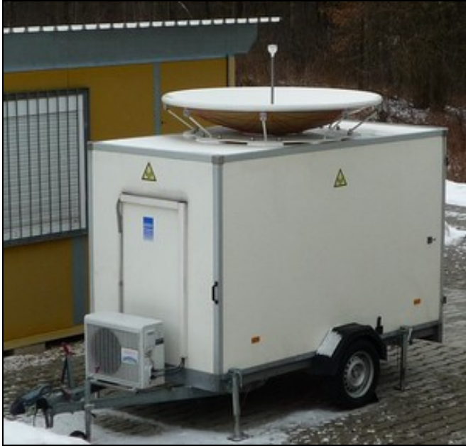
35 GHz cloud radar MIRA 36 from METEK
